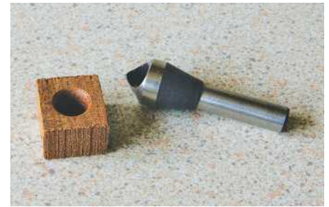
▲ Pic.12 Clean out the burrs from each side of the blocks and mount on a compression mandrel...
